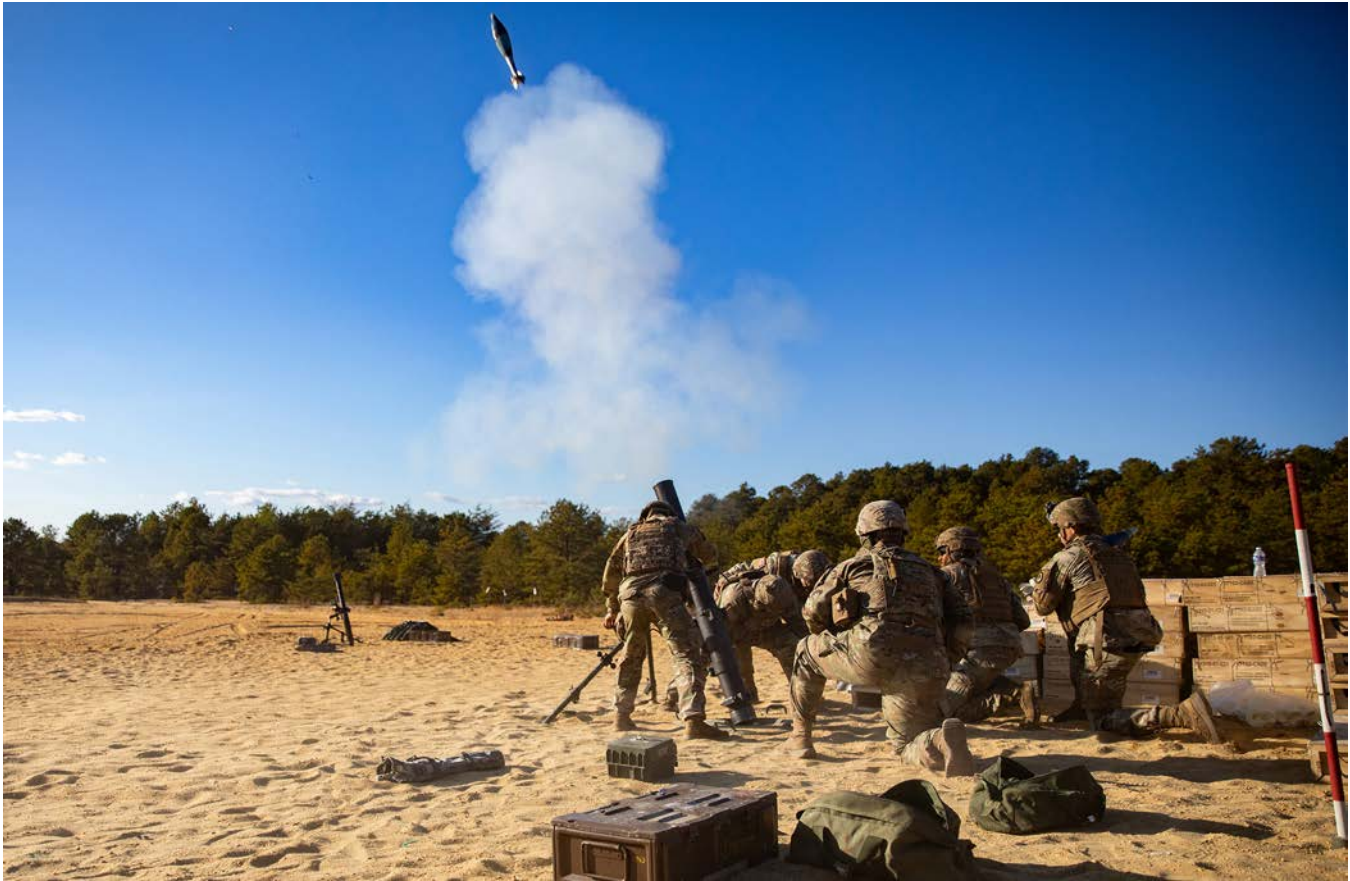
Above: Soldiers with the 114th Infantry Regiment prepare to fire a M121 120 mm mortar. The cannon, bipod, and base plate weigh 319 pounds.
